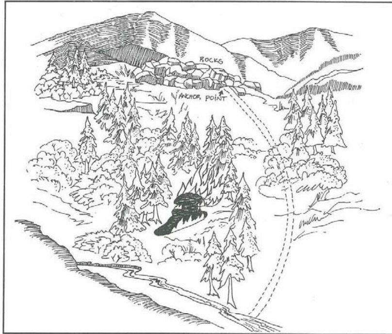
Figure 9 – Building Fireline Downhill
